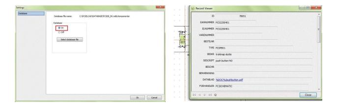
When the database is connected you can right-click on a symbol in the diagram, click Open and that way access the component database and get more information about the components.
