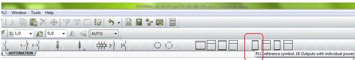
Plc symbols in this pickmenu are paired: two sets of inputs and two sets of outputs. You can see the descriptions for each symbol if you place the mouse on top of it. The difference is with or without individual power.
